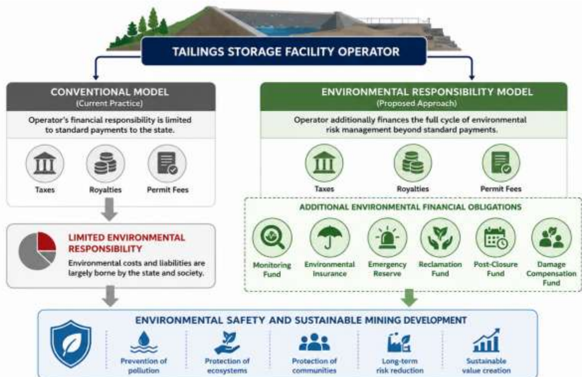
Figure 1. Comparison of conventional and environmental responsibility models for tailings storage facility operators. The proposed model requires operators to finance environmental costs associated with the prevention, monitoring, control, and remediation of current and future risks.
