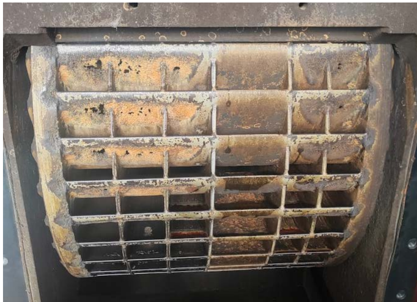
Fig. 2 Wear of the Crossflow turbine runner as a result of the ingress of large sediment particles
