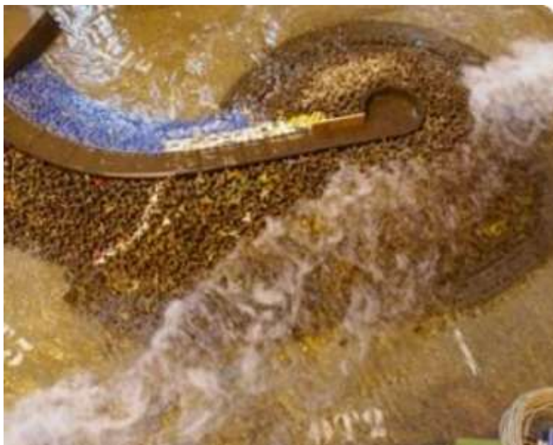
Fig. 11 Wave propagation on the outfall structure of the Safi thermal power plant (Morocco) - Scale: 1:68 [1]
