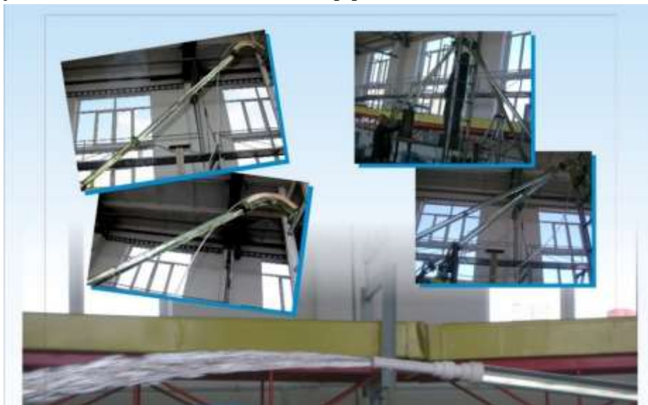
Fig. 20. Experimental setup for studying air accumulations in the hydraulic laboratory of the Institute of Water Problems and Hydraulic Engineering named after Academician I.V. Yegiazarov
