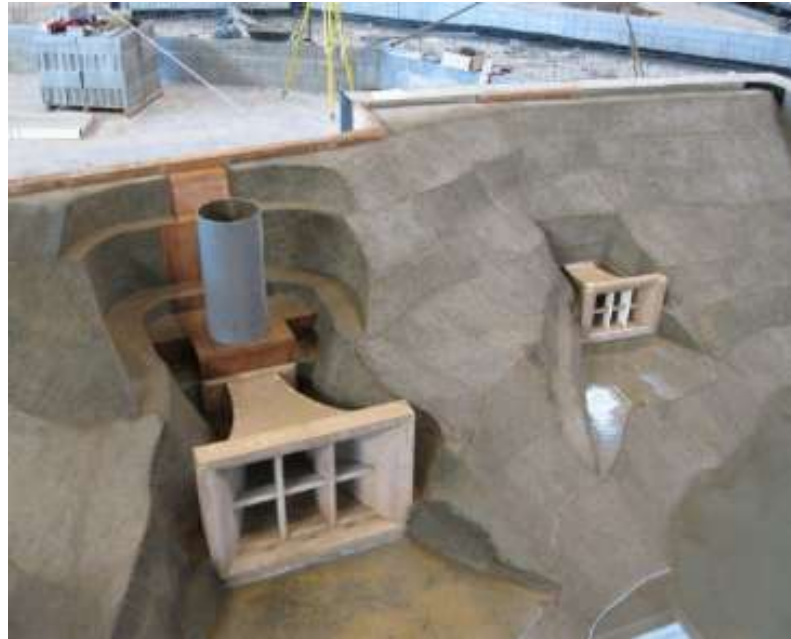
Fig. 12 Upstream water intakes of the Venda Nova III (pumped storage) hydropower scheme (Portugal) - Scale: 1:33.33 [1]
