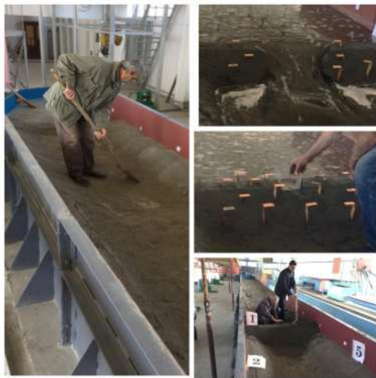
Fig. 17 Model of the collapse of an earthen dam in the Hydraulic Research Laboratory of the Institute of Water Problems and Hydraulic Engineering named after Academician I.V. Yeghiazarov
