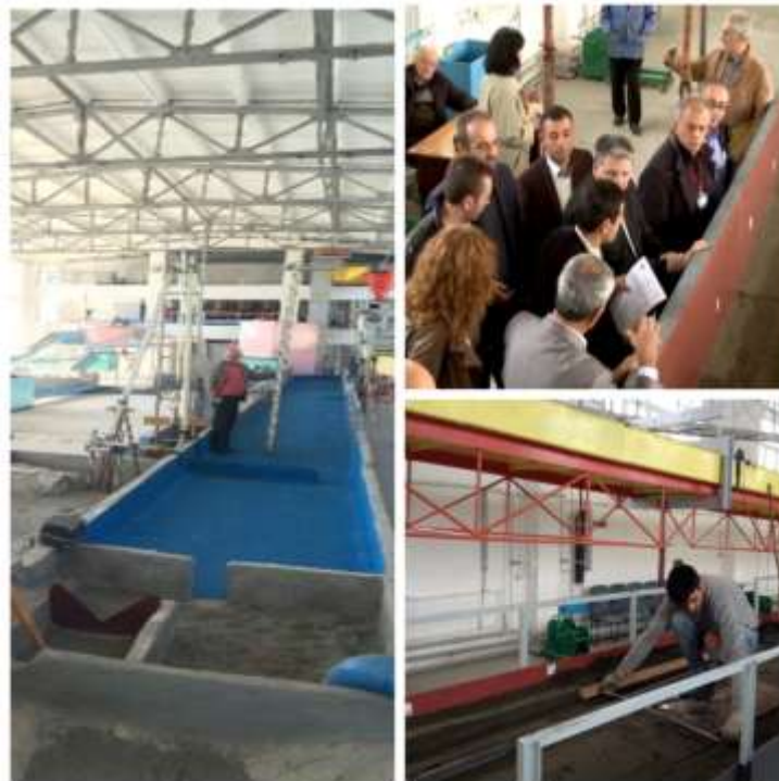
Fig. 19. Model studies of erosion of accumulated sediments in the hydraulic laboratory of the Institute of Water Problems and Hydraulic Engineering named after I.V. Yrgiazarov (within the framework of the European program: Greece, Turkey, Georgia, Armenia)
