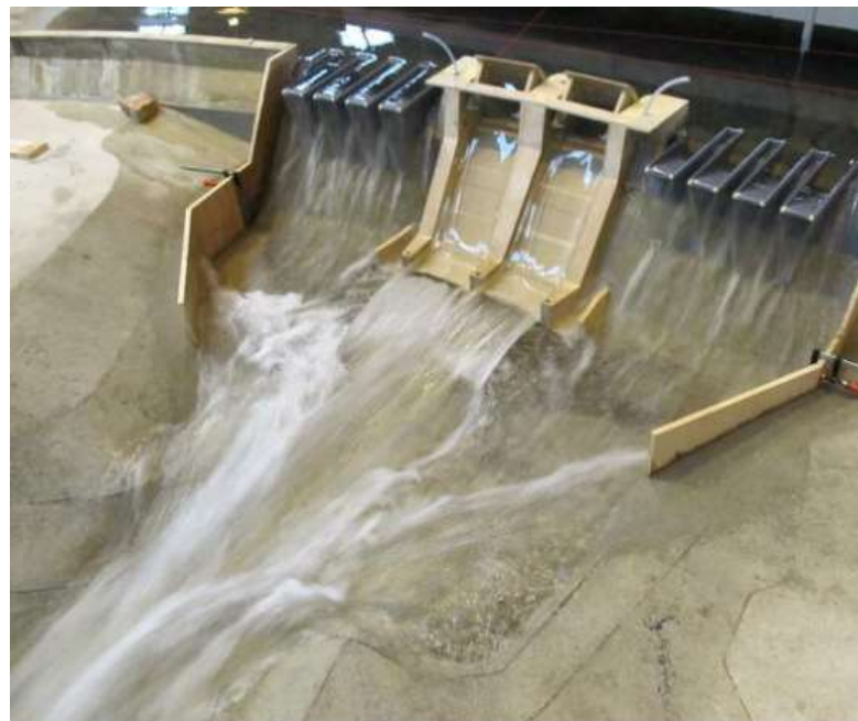
Fig. 14 Development of piano-key weirs on the existing spillway at the Charmine dam (France) [1]
