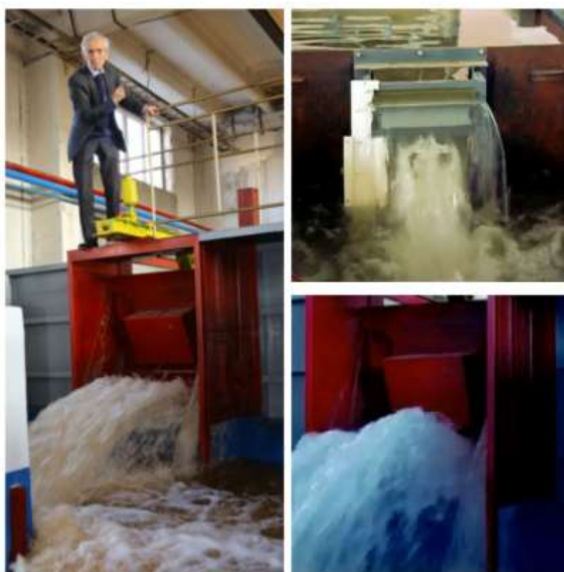
Fig. 15. Testing of the model and prototype of a stationary automatic gate in the hydraulic laboratory of the Institute of Water Problems and Hydraulic Engineering named after Academician I.V. Yegiazarov
