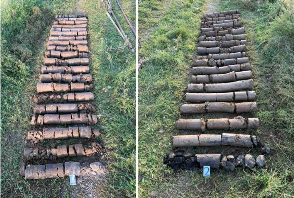
Fig. 4 Drilled cores from the second well (Left - cores at the beginning, Right - cores at the end)
