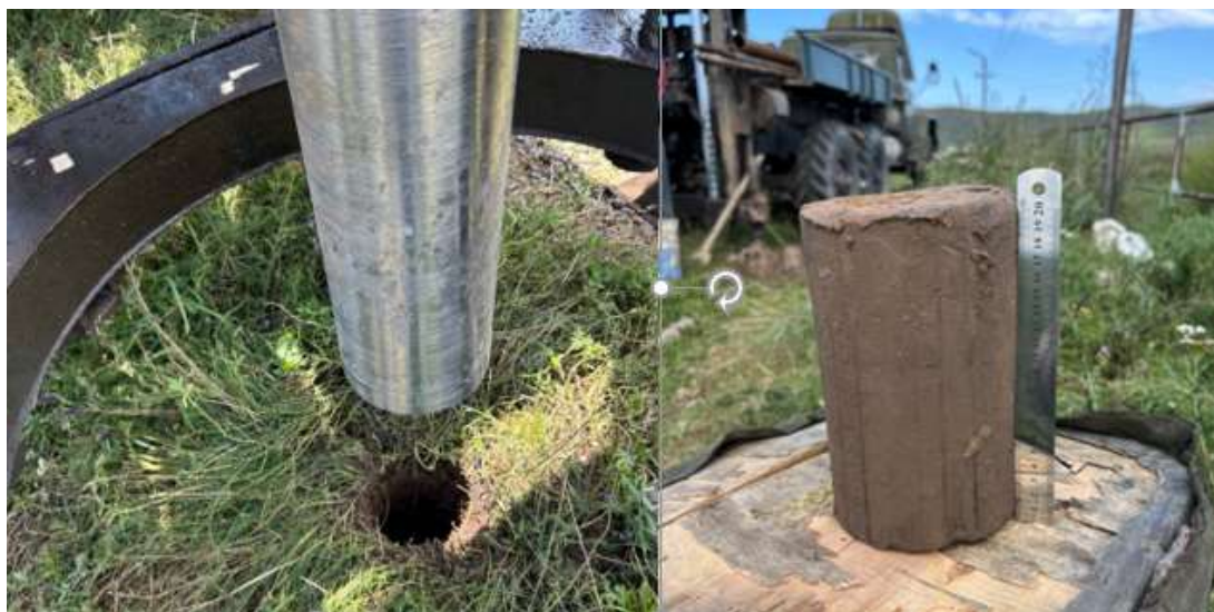
Fig. 2 Samples of natural state (monolithic) soil of the dam body «Gegharkunik 2»
