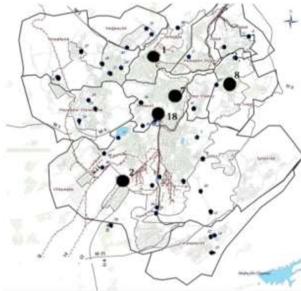
Fig. 3 Stationary (large black dots) & Mobile (small black dots) Observation Stations for Atmospheric Air Quality Monitoring in Yerevan[8]
