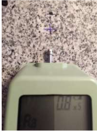
Fig. 5 Measurement of roughness distribution
